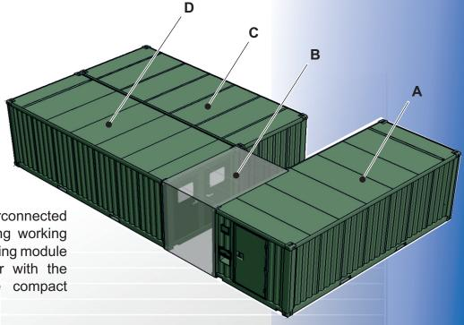
The laboratory is interconnected with entry and monitoring working place by the interconnecting module and it creates, together with the connecting cables, the compact MPML working place.
