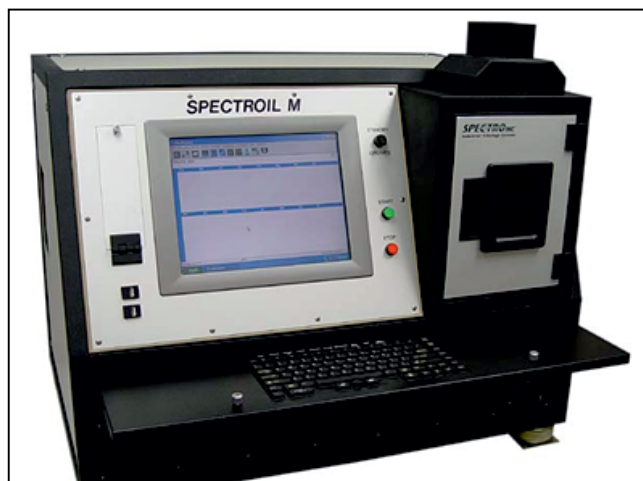
SPECTROIL M atom emission spectrometer with rotating disc electrode.
