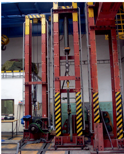
Binding equipments and ropes – loading stand for tensile tests
