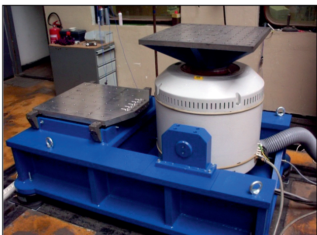
Mechanical resistance against the vibration and shocks - TIRAvib 57315 LS
