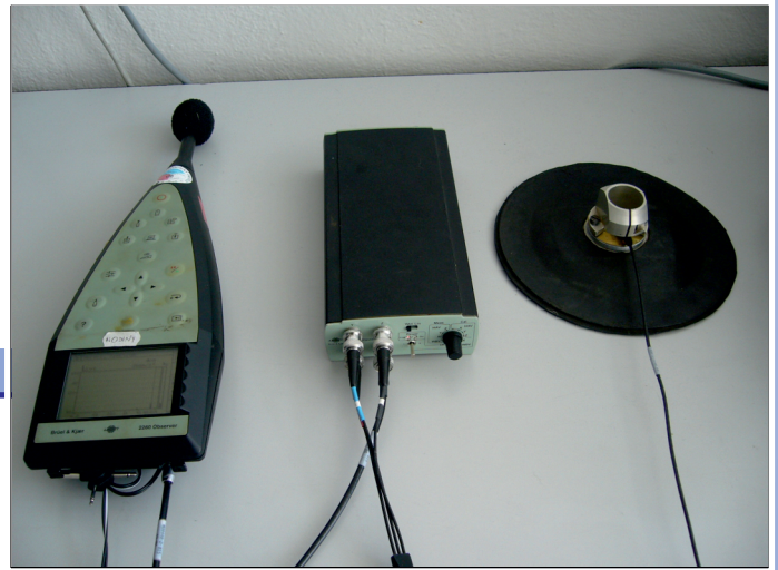
Vibrations affecting the human body - Vibrometr B&K 2260 Observer
