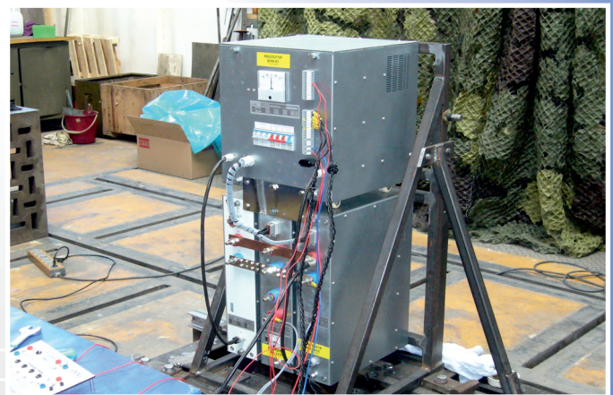
Tests of mechanical resistance of locomotive blocks
